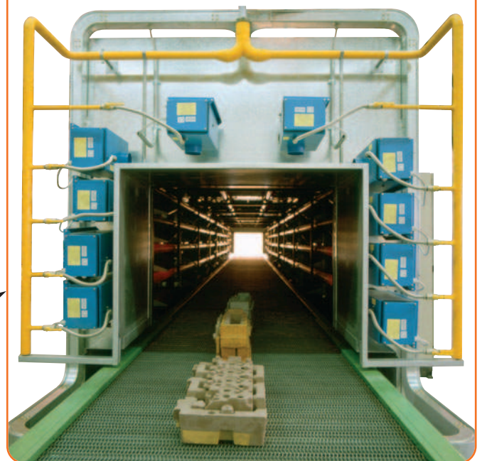
Example of a drying installation for water paintings on foundries souls.
