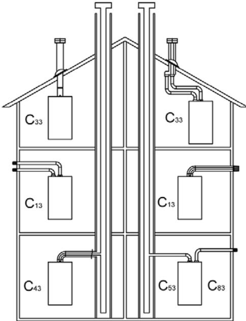
**Configuration C13:** Air/flue gas connection by means of concentric pipes to a horizontal terminal or twin pipes in the same side (so called forced flue)
